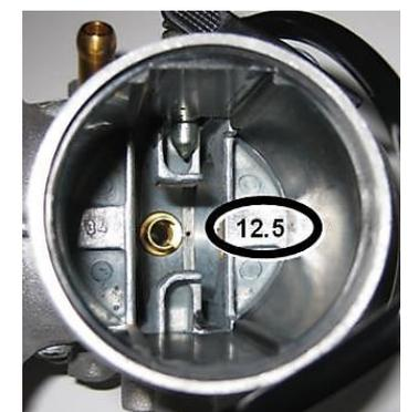
Angular bore of carburettor insert. Plug gauge 0,60 must not enter the bore (use jet gauge set ROTAX 281 920).
