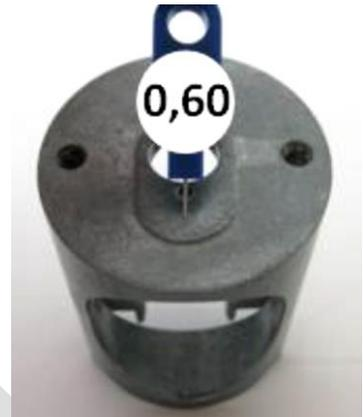
Vertical bore of carburettor insert. Plug gauge 1,30 must not enter the bore (use jet gauge set ROTAX 281 920).
