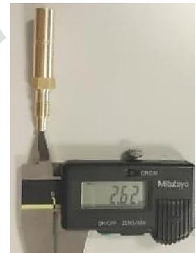
Idle jet must be stamped with "60". Plug gauge 0,65 must not enter the bore (use jet gauge set ROTAX 281 920).
