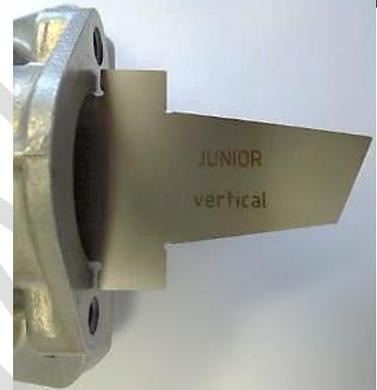
The template must be moved in horizontal and vertical Position as far as possible into the exhaust port.
