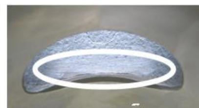
The exhaust port may show partial manual grinding done by the manufacturer to eliminate minor casting defects and/or to eliminate the NIKASIL burr at the end of the NIKASIL plating (see above right picture).
