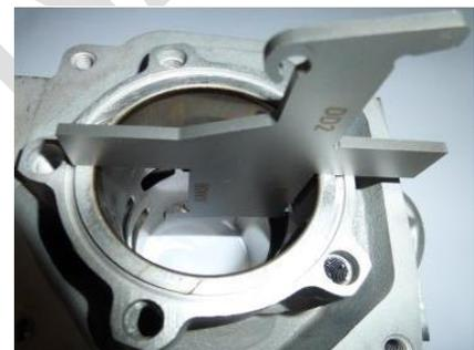
Insert the template into the cylinder and move the template (at the highest point of the exhaust port) as far as Possible into the exhaust port. In this Position the template may not touch the cylinder wall.
