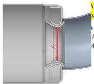
A solid flat plate measuring 28.0mm and 1.5mm thick **must not** pass through Section "A" and
